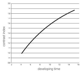
Evolution of the contrast index of Print Film as a function of processing time in D76 stock (22°C)
